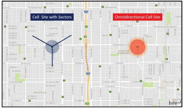
Figure 1. Omni-Directional vs. Sectorized Cell Site Example
